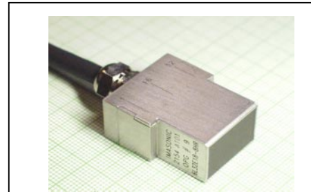
Probe 09: 6L32E18-8HR 32 elements / 0.55 mm / 6MHz
