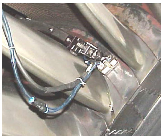
Fig. 10: L-0 steeple inspection with 3-heads probe
