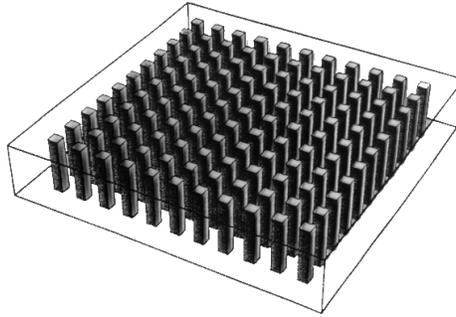
figure 6. Schematic representation of a piezo-composite plate with a 1-3 structure - After W.A. SMITH
