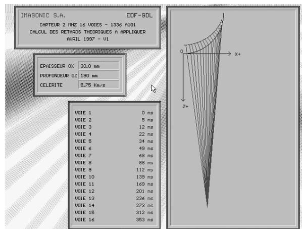
figure 5. Delay laws calculation software
