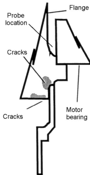
figure 1. cracks to be detected
