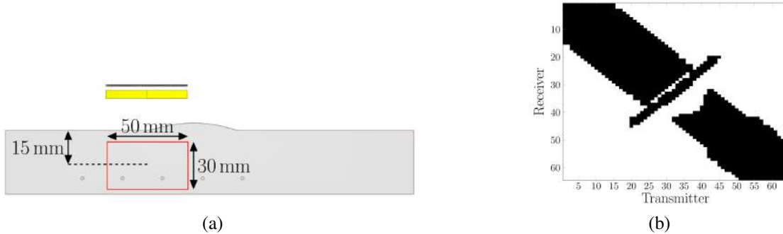
FIGURE 10. Weld bead. (a) specimen geometry, (b) K(t) matrix with a threshold at -6 dB.
