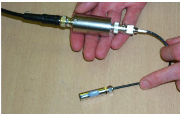
**FIGURE 1** : single element transducer and external matching circuit
