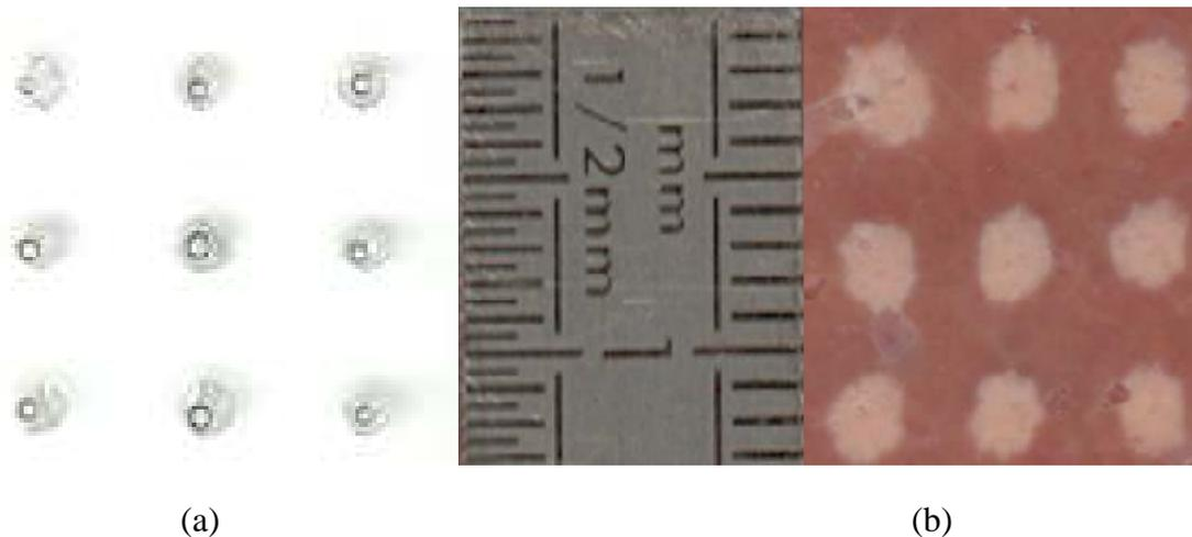
**FIGURE 6.** a) Impacts induced in a slice of plexiglas located in the focal plane ( $Z = 120$  mm) through the skull. The impact size is about 2 mm. Aberration corrections were achieved at center by using an hydrophone and next impacts were achieved by tilting electronically the beam. b) same experiment on liver.
