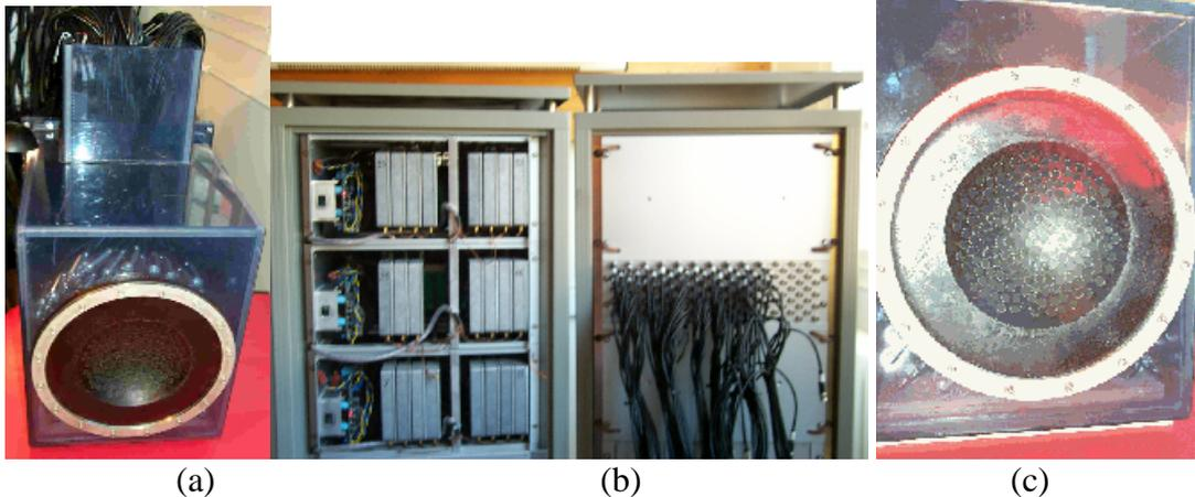
**FIGURE 4.** (a) 200 elements sparse array prototype and the electronic system. The waterproof plastic box contains the 200 electrical matching boxes. (b) High Power electronic (individual channels) Quasi random distribution of transducers embedded in spherical shaped Ureol. (c) Front view of the array: the transducers are mounted on a spherical surface.
