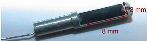
**FIGURE 1.** A dual mode transducer
